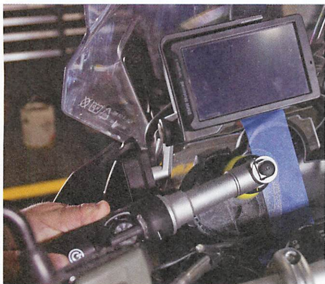
The Bigfoot iBrid Nano polisher can reach into tight spaces, like a big electric toothbrush (left). Half of the gauge cluster was masked and polished. The difference can clearly be seen (above).
