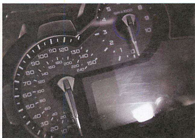
The Bigfoot iBrid Nano polisher can reach into tight spaces, like a big electric toothbrush (left). Half of the gauge cluster was masked and polished. The difference can clearly be seen (above).
