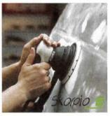
low vibration levels. It's available in either 3 mm or 6 mm orbit. A new multi-hole slim backing pad maximizes dust extraction on both horizontal and vertical surfaces.
